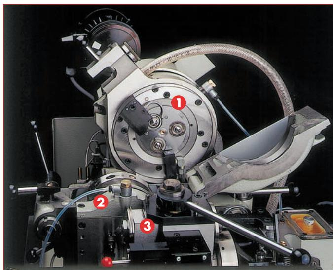
1. Turret (D5) with counter collet and 2 drilling spindles
